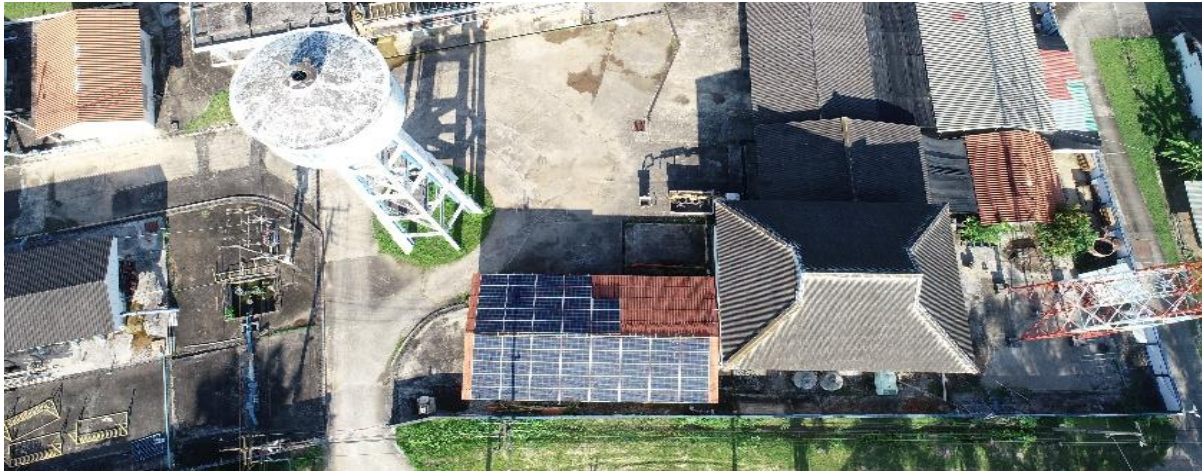
Solar panels with 20 -kW installed capacity on the roof Water production building
