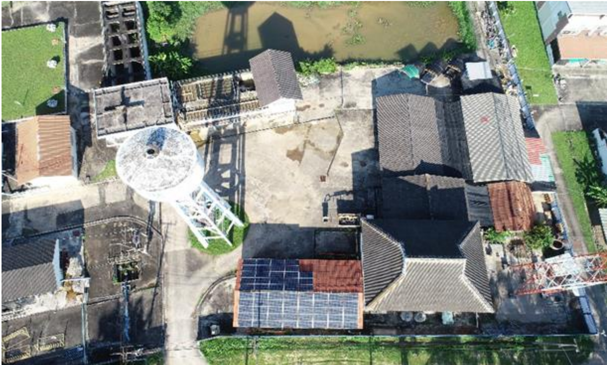
Solar panels with 20 -kW installed capacity on the roof
