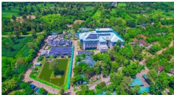
Solar panels on the roof of the School of Renewable Energy have a capacity of 660 kW
