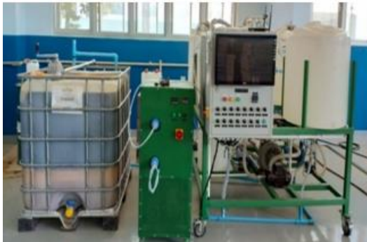
Biodiesel plant with a 150-liter-per-batch capacity made from cooking oil waste and oil plants.
