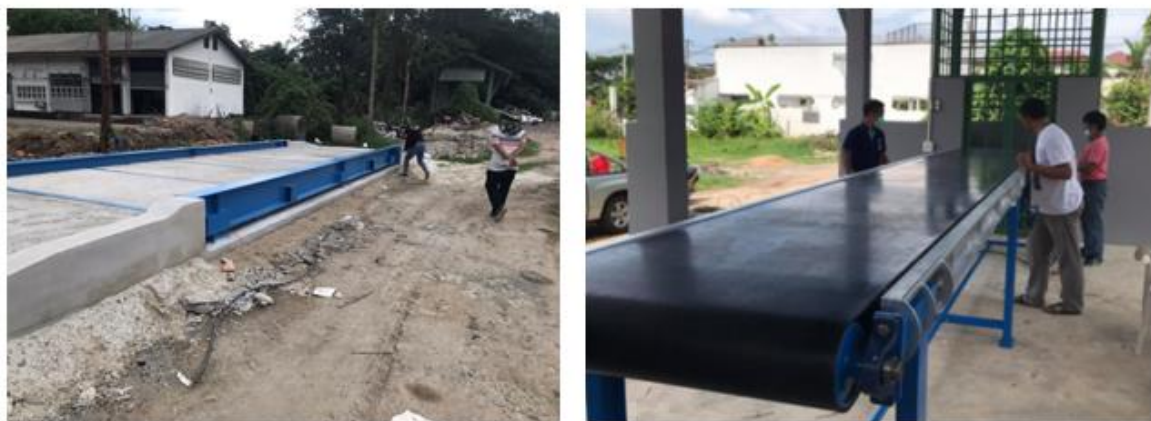
Weighting scale and conveyor were installed at the MJU recycling center
