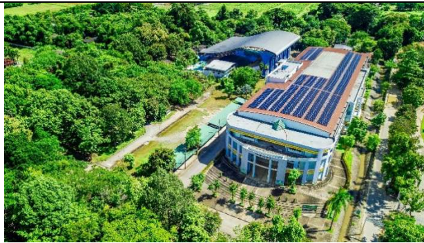
Solar panels with 40-kW installed capacity on the roof, Umuay Yodsuk
