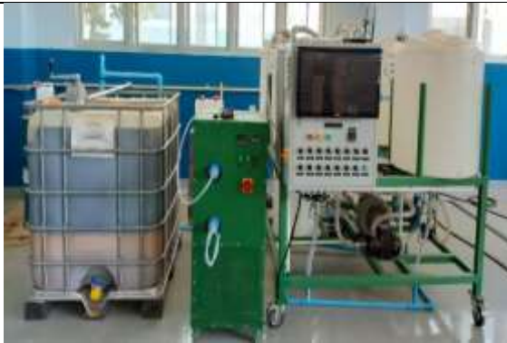
Biodiesel production system capacity of 150 liter from wastes cooking oil and oil plant
