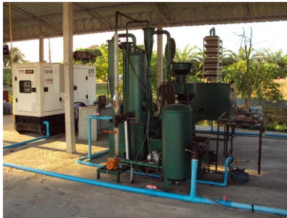
Biomass gasification for power generation 30 kW
