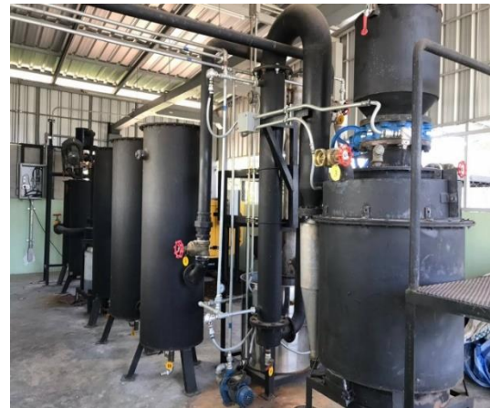
Biomass gasification for power generation 20 kW
