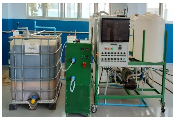
Biodiesel production system with the capacity of 150 liter from wastes cooking oil and oil plant
